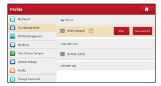
If several VCI devices are activated on this tool, a list of VCI devices will be displayed on the screen. If your tool extends to support heavy-duty trucks, you need to switch to the corresponding VCI module before diagnosing it.
